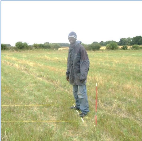
Two other pieces of equipment are used to help us carry out our survey: A 'trapeze' which comprises two poles (we use plastic piping) with washing lines at each end which extend the full length of the grid. The lines are marked at 1m intervals to help us pace ourselves as we walk with the magnetometer.
